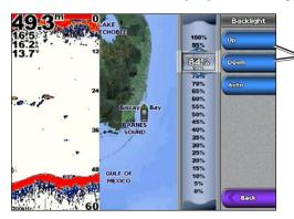
To manually adjust the backlight, either select **Up** or **Down**, use the **ROCKER** (GPSMAP 4000 series), or touch and drag the brightness bar (GPSMAP 5000 series).
